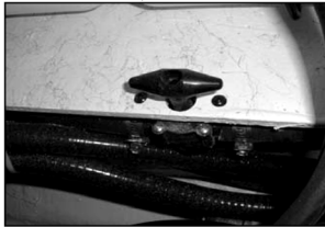
Fish box drain valve on model 2300. Located in battery compartment
