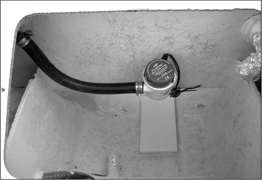
Fish box drain valve on model 2300. Located in battery compartment
